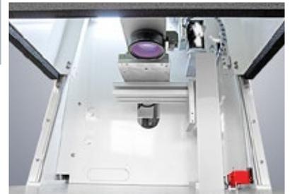
**MicroMark G3** has been developed with a vertical door on three sides so as to guarantee quick and convenient access to the marking compartment. Furthermore, by wearing safety goggles and working with the door open you can also mark large details using a machine that is just slightly larger than a small desk.
