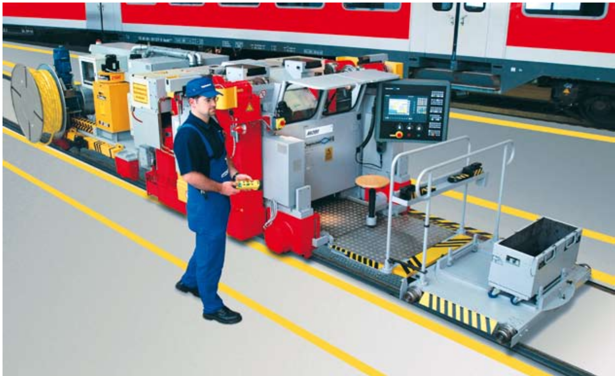
MOBITURN ® - the mobile wheel set reprofiling facility
