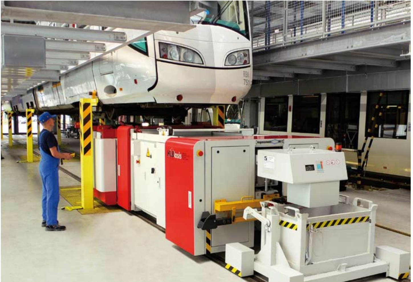
The first and only mobile wheelset reprofiling system
