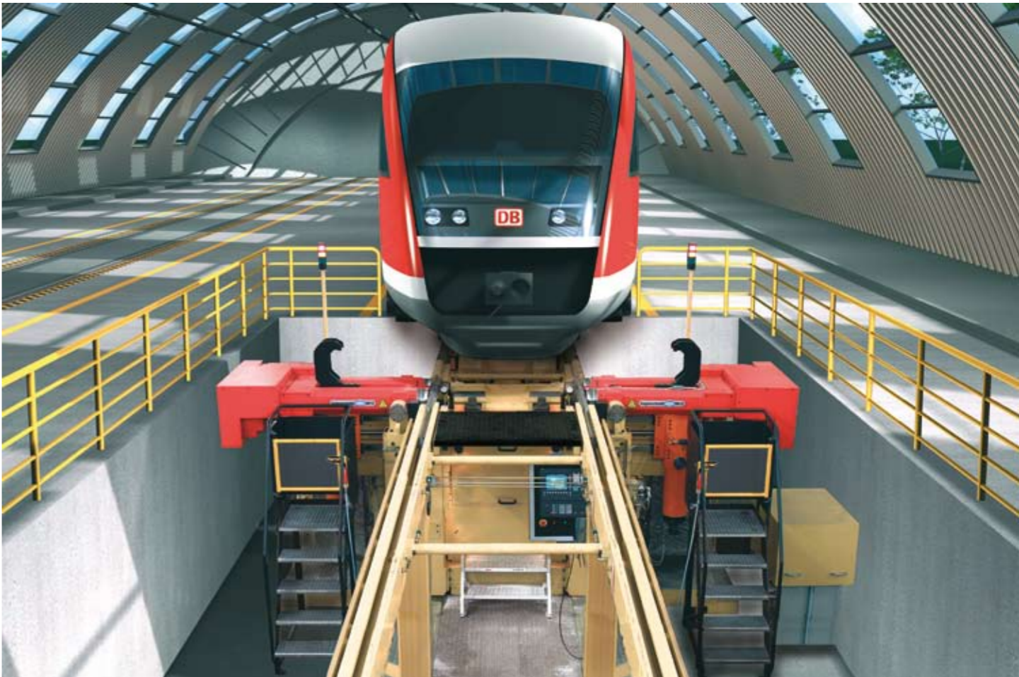
CNC-controlled machine with automatic measuring system
