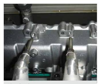
**Adapted nozzles** for targeted inside cleaning of borings
